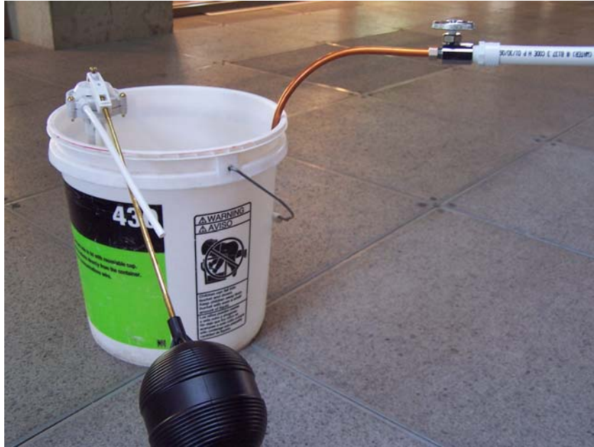
Figure 6: Mechanical Float Switch Design
